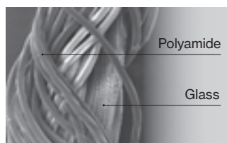
Solid construction. Core – shell – thread.
