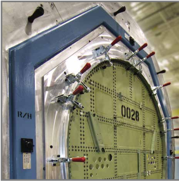
Model 210-U used in an airframe assembly fixture
