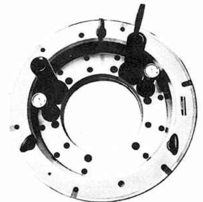
Broaching of turbine blade components on the CFM 56 (SNECMA) drum
