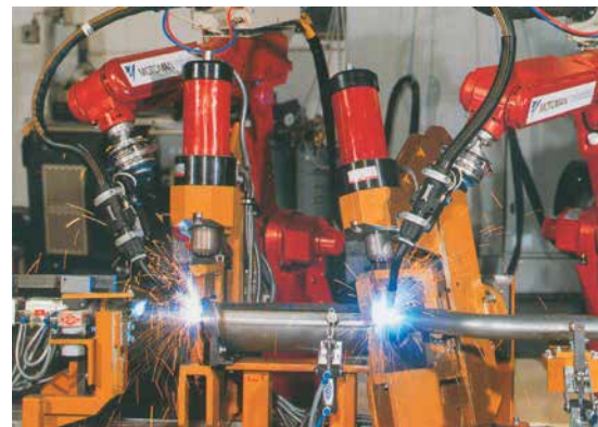
Welding fixture for exhaust components
