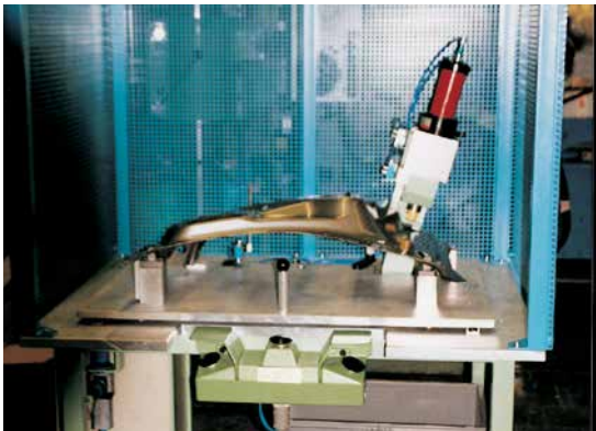
Device for holes Ø 8 in sheet metal
