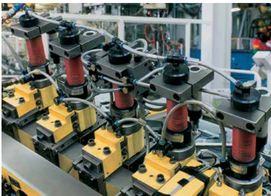
Stamping units placed in line
