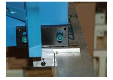
Name: Blue Slice Nest Tooling Material: Blue Nylon, 1" (25.4mm) thickness Benefits: Lightweight, durable, machinable material Process: Machined from 3D CAD
